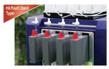
8. Install all T-locker valve on each cartridge (Horizontal position means close and vertical position means open)
