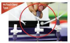
9. Cut an ink tube with proper length from 1 liter ink pouch stand and connect an ink tube to each T-lock valve.
