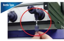
3. (Remove the front cover if needed.) Fit an ink tube with a connector and fit it with O-ring. Then place and push it to the end, and fasten the connector with hand. (refer to 2-1 How to connect an ink tube)
