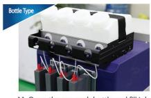
11. Open the cap each bottle and fill ink into each bottle with its corresponding color.
