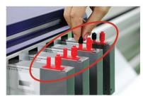
1. Plug each cartridge on a printer and remove a black cover.
