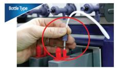
4. Cut a ink tube with proper length from the bottle and connect an ink tube to a cartridge with same way of connecting it to bottle. (refer to 2-1 How to connect an ink tube)
