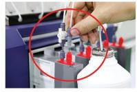
13. After filling ink in cartridges, slightly unfasten an air removal cap and put a suction needle in it to remove air, then fasten the cap.
