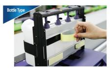
2. Detach the paper from the bottom of a bottle unit and place it on the preferable location.
