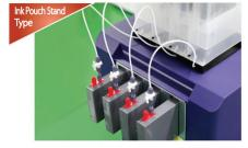
12. Put the 1 liter bagged ink in the case and plug it to each stand with its corresponding color and open the T-valve to let ink supply to cartridges.
